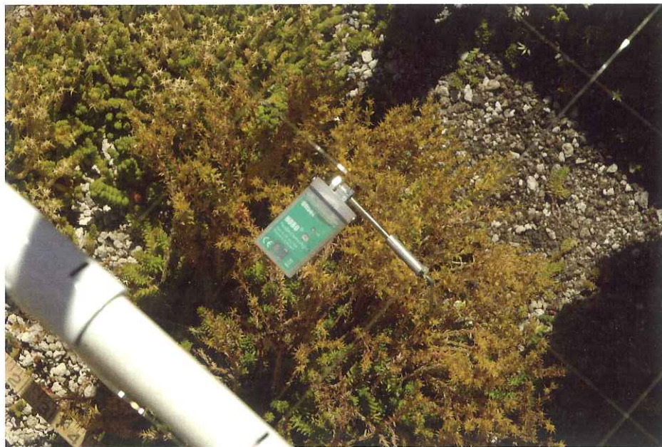
Data loggers arrayed above the plants automatically record air temperature and light every 30 minutes. Additional sensors buried beneath the soil measure how the plants and substrate affect the temperature of the roof below.
